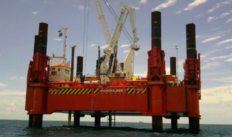
LEFT: Van Oord's 'Wavewalker' drilling and blasting platform used to blast the rocky sea bottom. Photo: Both ENDS, 2014. RIGHT: Marisqueiras at work in Suape port area, with shipyard in the background. Photo: Both ENDS, 2014.
